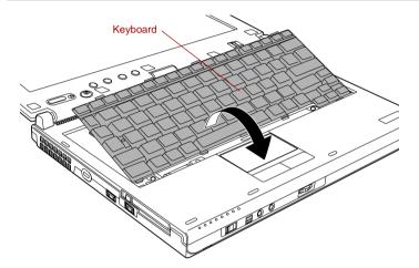
Figure 3-9 Rotate the keyboard
